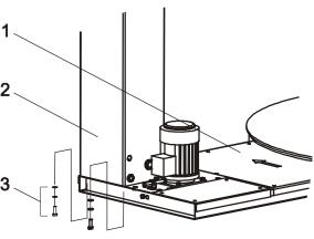
proper places of the machine in production. Remove them and erect column pos. 2 (carefully to prevent damaging of cables; the mass of the column is equal to 85 kg to 95 kg, according to the outfit) and screw it to the turntable pos. 1 by screw stock pos. 3 - it is screwed to the column from below. When the column is erected, the handling fixture has to remain in its place.
