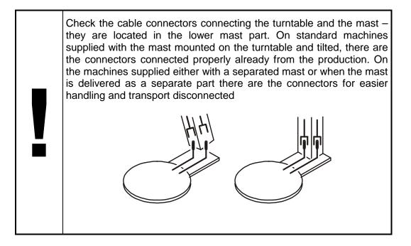
After a careful check of the connection the plug may be inserted in the socket and the machine may be connected to the mains by the main switch.
