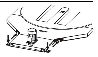
• Footings fastened to the turntable. During manipulation they lean from the bottom against the skids of the high-lift truck.
