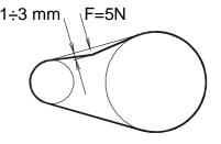
should the chain bend by 1, max. by 3 mm. If necessary to adjust the distance of axis proceed as follows: upper bearing of main roll is inserted in a box with enlarged holes. When removing the bolts the box may be shifted and thus adjusted a correct chain tension. Do not handle lower bearing of main roll any way, a slight abberance does not inluence neither the functionality not the reliability of device. Tighten the bolts finally.
