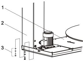
proper places of the machine in production. Remove them and erect column pos. 2 (carefully not to damage cables; the mass of the column is equal to 85 kg to 95 kg, according to the outfit) and screw it to the turntable pos. 1 by connecting material pos. 3 – it is screwed into the column from below. When the column is erected, the handling fixture has to be left in its place.
