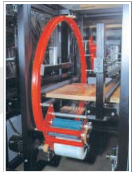
The prestretching device for increasing the wrapping quality, lowering the packaging price and foil consumption by 20 - 30 %. This secures a fast rate of return of investment.
